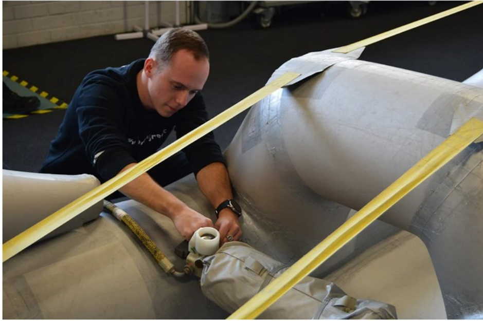
Cabin evacuation slides must undergo annual inspections starting at 15 years after manufacturing. Credit: Magnetic Group
