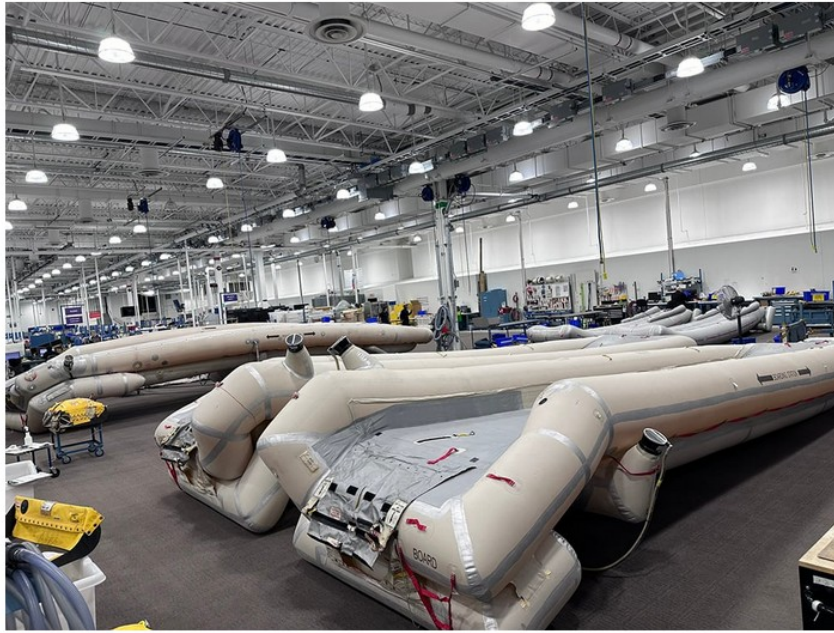
Escape slides typically stay on-wing until scheduled maintenance is due. Credit: AJW Technique
