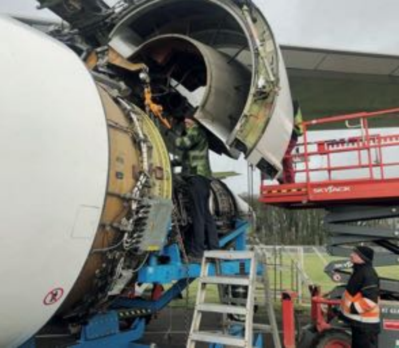
After removed parts have been inspected and cataloged into the system, their condition is assessed for serviceability and their potential resale value, says AJW's Tony Whitty. AJW image.
